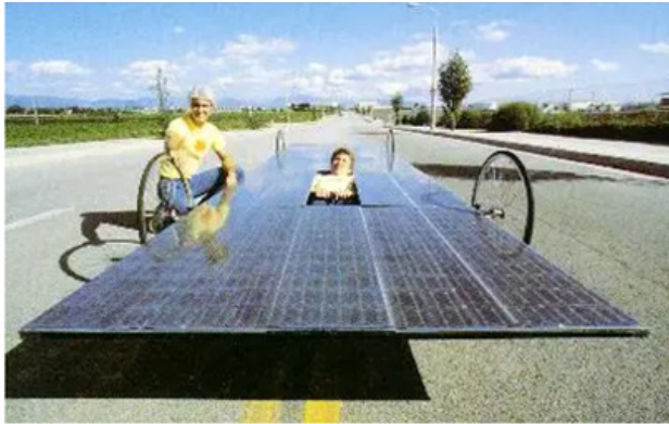
Sunrunner 1.2kW solar arrav (no batteries)
