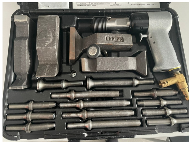
Figure 10. Pneumatic Riveting Gun Set
