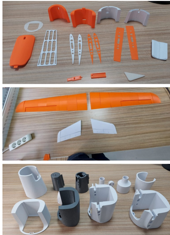
Figure 7. 3D printed wing, tail, and fuselage components
