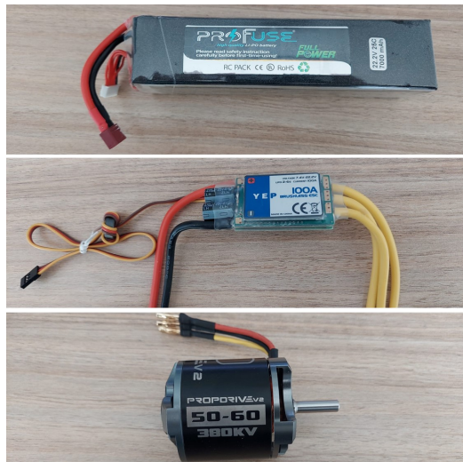
Figure 6. Propulsion system components: Battery, ESC, and motor
