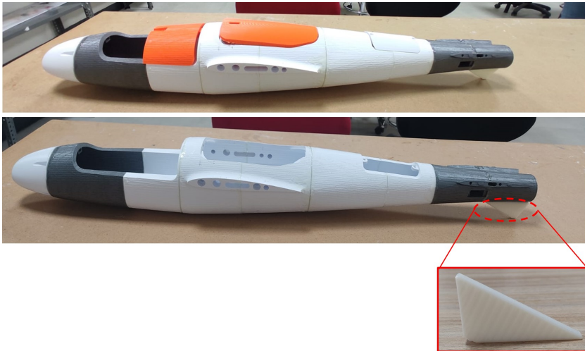
Figure 8. Fuselage and fin structure bonded with epoxy resin
