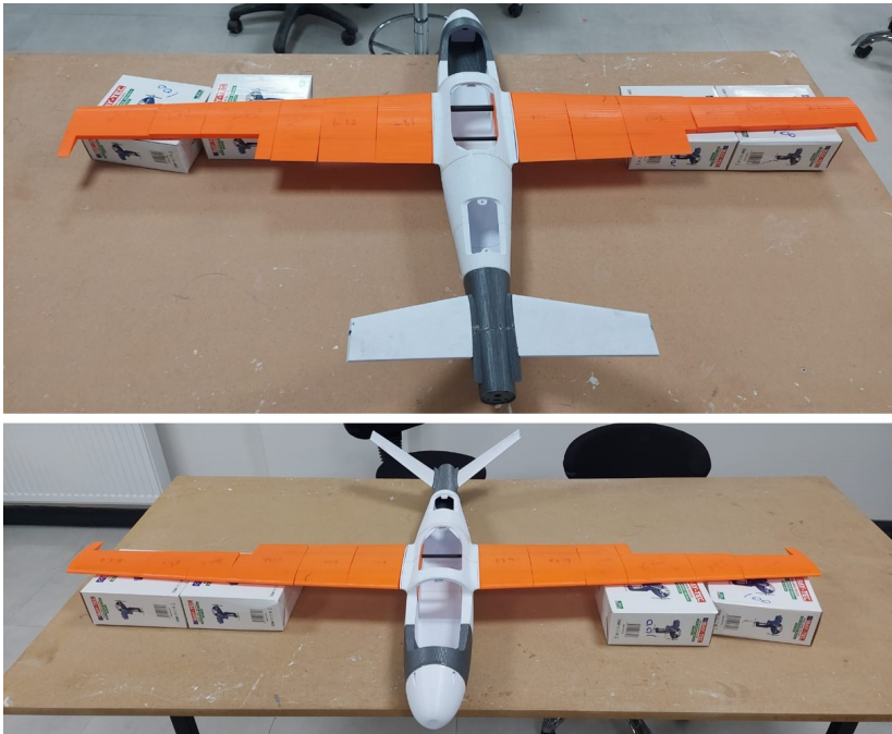
Figure 9. Rear and front views of the manufactured UAV after wing and tail assembly
