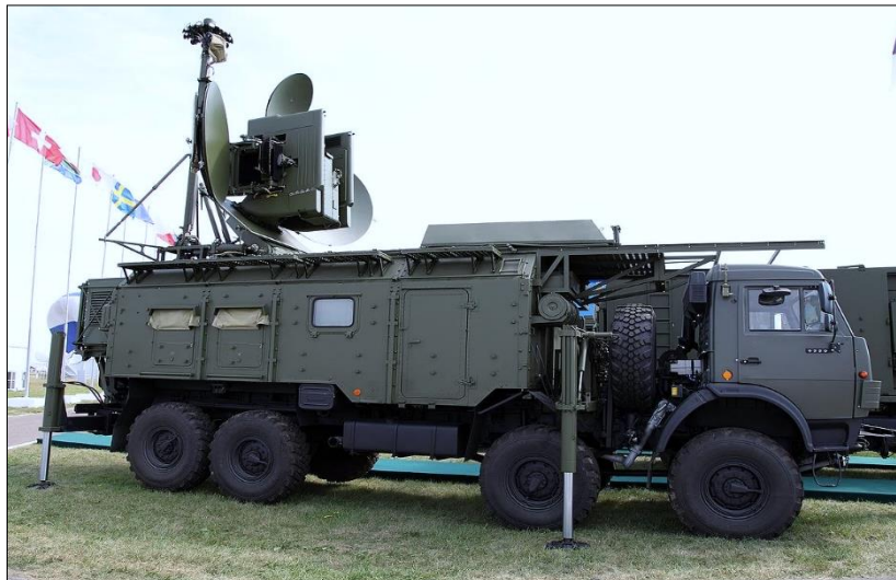
Figure 11. Ground-based electronic suppression module 1RL257E Krasukha-4
