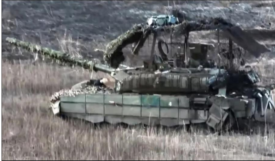
Figure 9. The abandoned T-90M with the drone jammer on top of the turret.[24]
