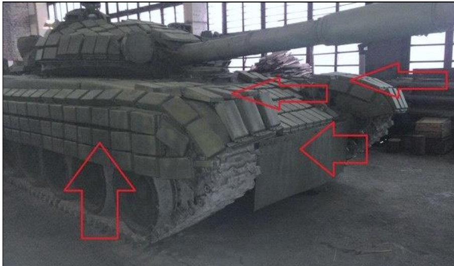
Figure 6. One of the radically modernized T-72B in Novorossia with dynamic protection on MTO
