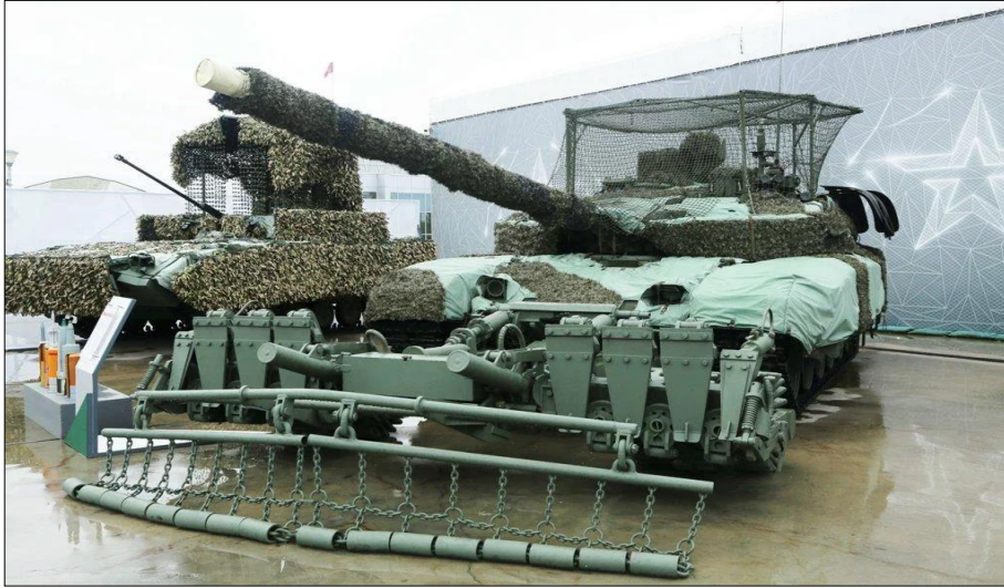
Figure 10. T-90M Nakidka Thermal Cover & Kits
