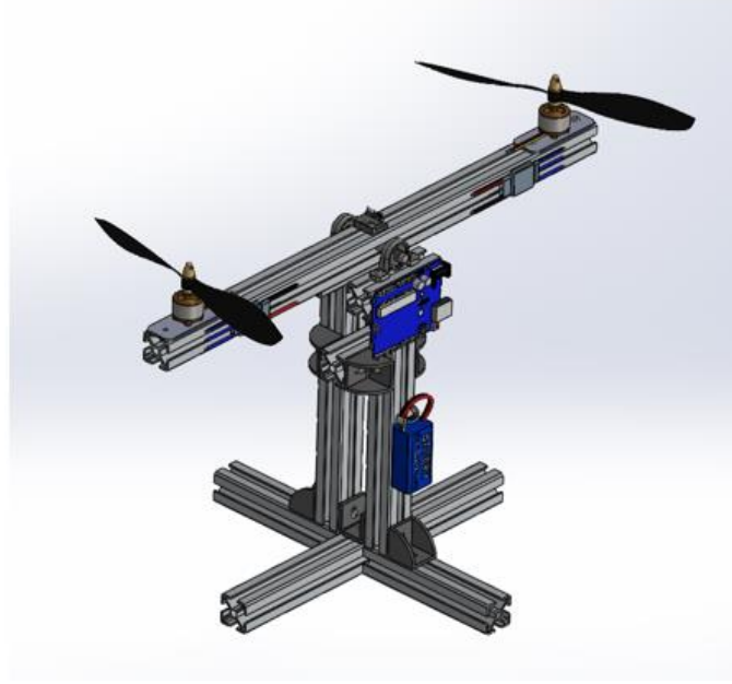
Figure 3. Designed Single-Axis PID Test Setup
