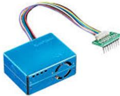
Figure 6. PMS5003 Digital Particle Concentration Sensor
