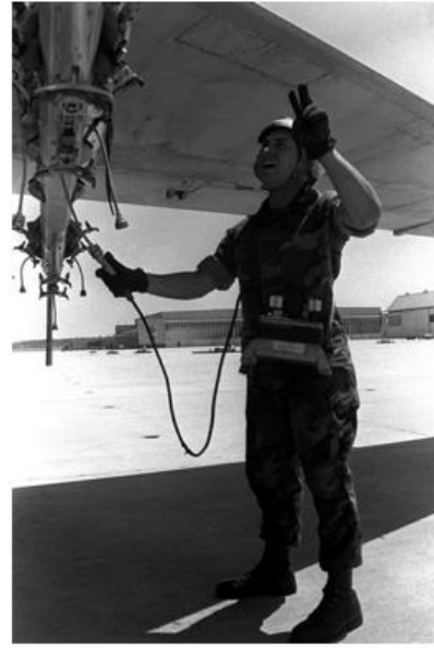
Figure 10. A member of Marine Attack Squadron 224 (VMA-224) pointing to the cockpit while using the AN/AWM-54 aircraft firing circuit test set to test the multiple launch rack (MER) on the wing of the A-6E Intruder aircraft
